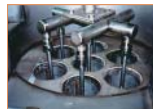
Rigid EZ Align™ discharge electrodes with tube type collecting electrodes
